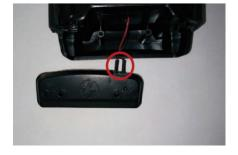
Last but not least, you disconnect the wiring off the rear light. Please pull directly on the contacts and not at the wiring!
