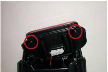
Now, you remove the two screws which fix the rear light tot he coverage.
